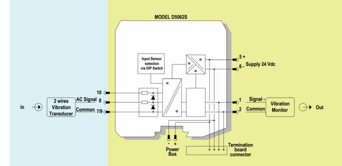
Input configuration selection via internal Dip-Switch
